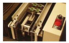
Versatile Heller in-line cure ovens transport standard to ultra-thin boards.
